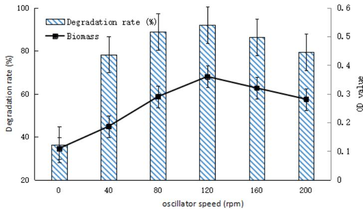
**Fig4. Effect of oscillator speed on chlorpyrifos-degrading rate**
