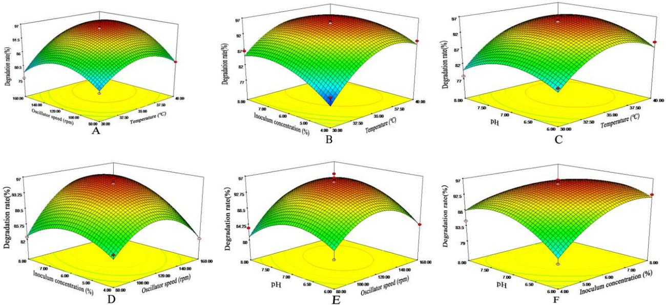
**Fig.6. The 3D plots showing the effects of variables chlorpyrifos-degrading rate.** (A) The interaction of temperature and oscillator speed. (B) The interaction of temperature and inoculum concentration. (C) The interaction of temperature and pH. (D) The interaction of oscillator speed and inoculum concentration. (E) The interaction of oscillator speed and pH. (F) The interaction of inoculum concentration and pH.
