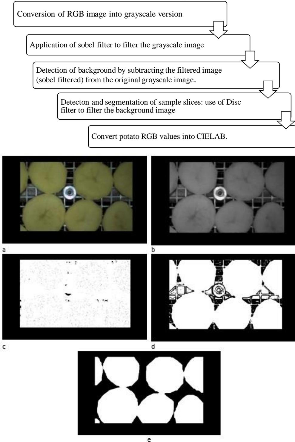
**Fig. 3** Steps involved in image analysis process for color data: (a) RGB image (b) grayscale version of image (c) filtered grayscale image (d) detection of background (e) segmented sample slice
