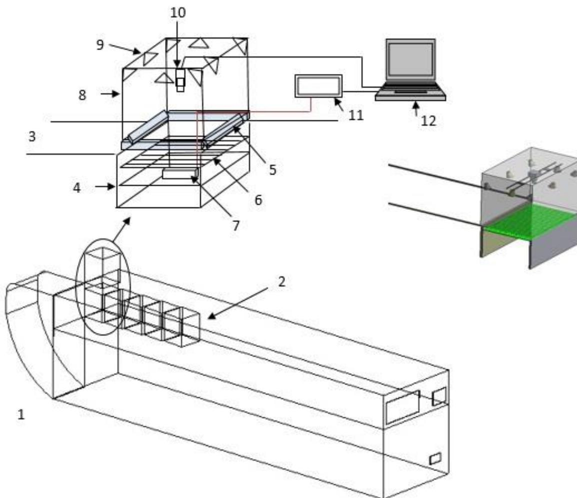
**Fig. 1** Real time data acquisition system. (1) Diagonal-airflow dryer (2) Food buckets arranged in diagonal form (3) roof of the dryer (4) Plastic bucket for food samples (5) Acrylic sheet (6) Food tray (7) Load cell (8) Imaging box (9) Florescent lights (10) imager i.e. camera (11) Data logger (12) Computer.
