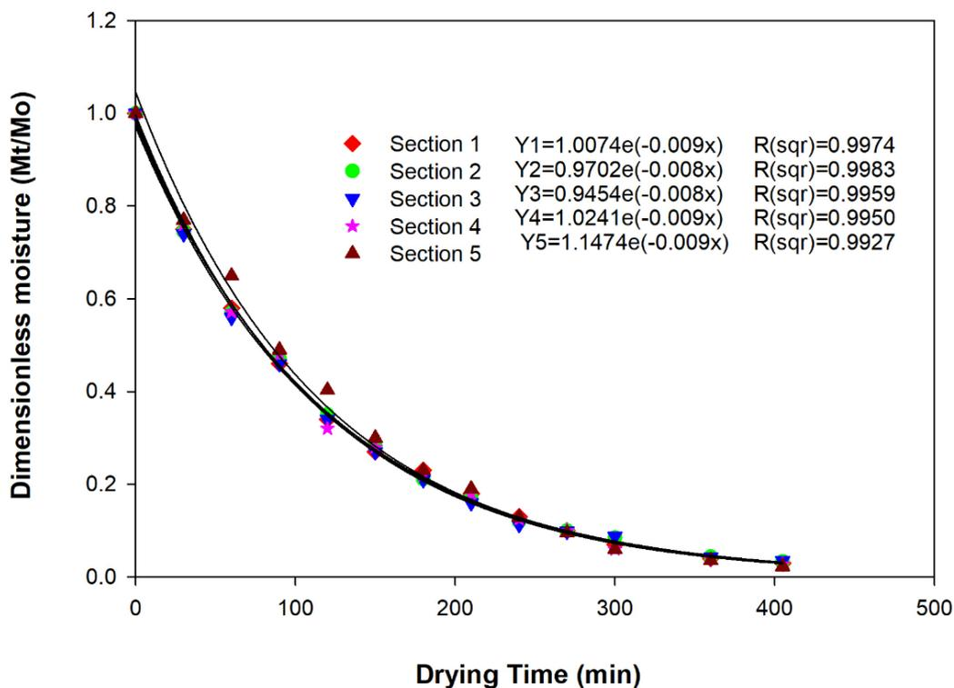
**Fig. 4** Drying characteristics of potato slices at different sections of the drying chamber
