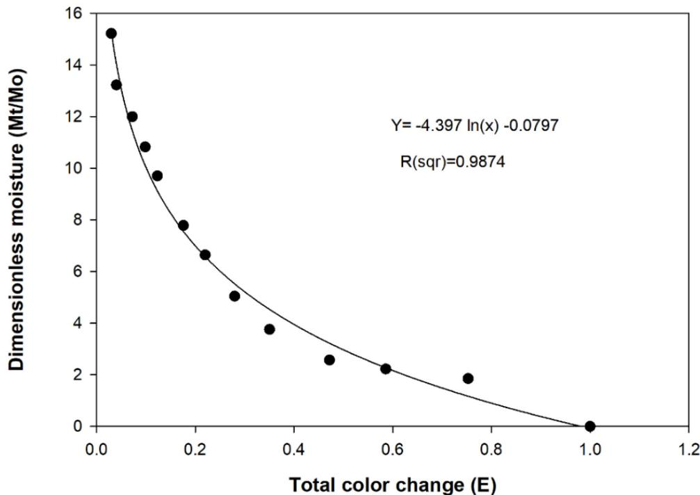
**Fig. 6** Relationship between experimentally measured moisture ratio and total color change
