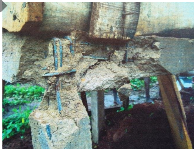
Fig 7: RC frame model near collapse
