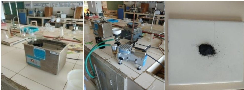
Fig 3. Sequential operations in MWCNT surface oxidation to form MWCNT-F
