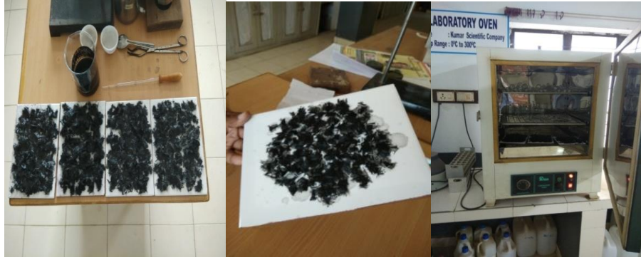
Fig 4. Grafting MWCNT-F on CF Surface
