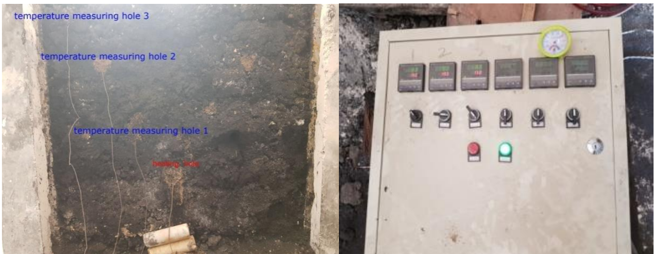
Fig.3 Heating layout of coal body
