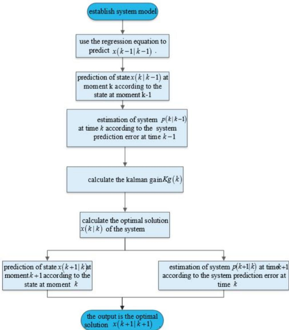
Figure 1: The flow chart of Kalman filter algorithm
