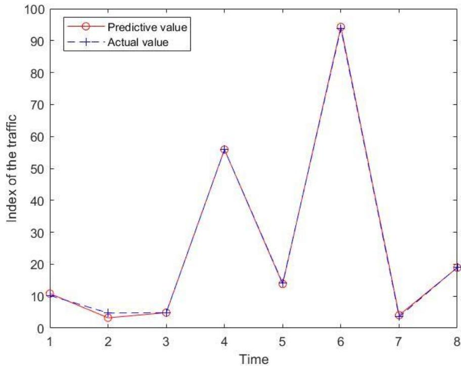
Figure 3: curve fitting the measured value of traffic index and the output value of BP neural network
