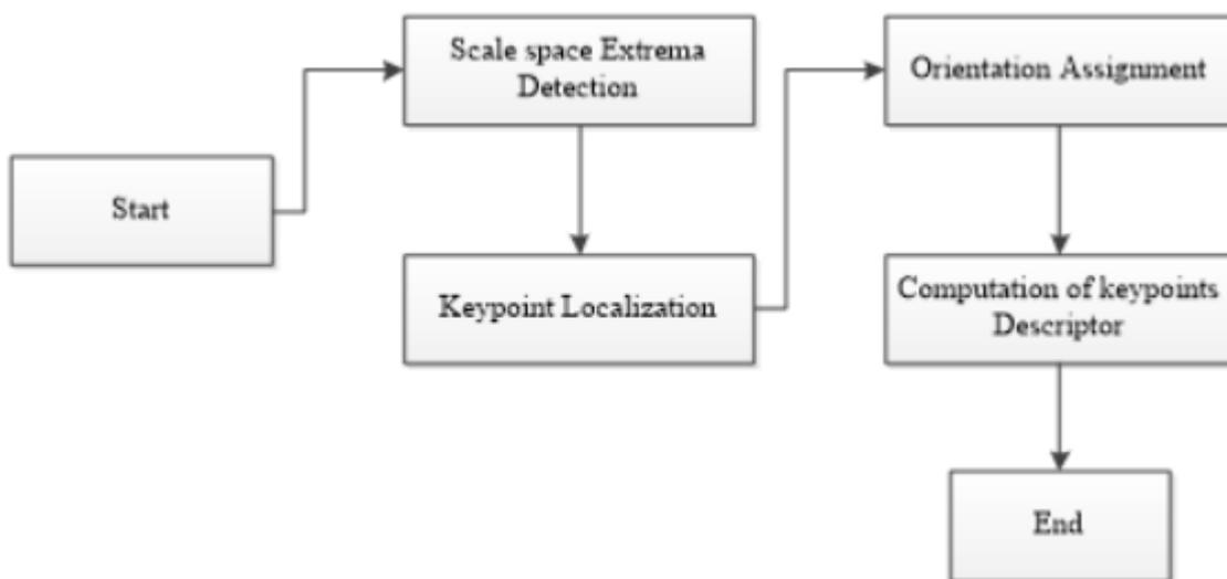
Figure 2: Block Diagram for SIFT
