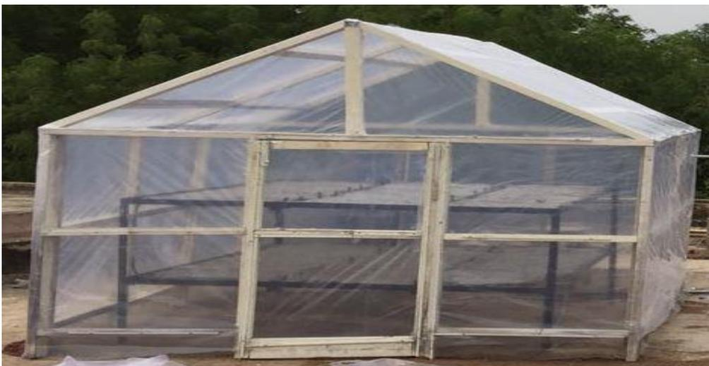
**Figure.2. (a)** Pictorial views of experimental setup, Mushroom drying in greenhouse under natural convection mode.
