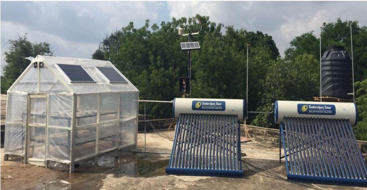
**Figure.2. (b) Pictorial view of Experimental setup, Mushroom drying in greenhouse under forced convection mode.**
