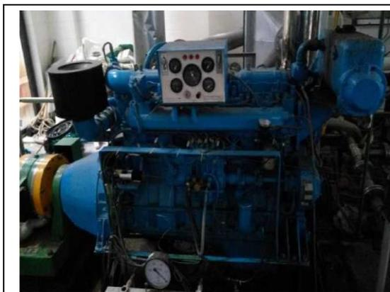
Figure 2. 6135 diesel engine
